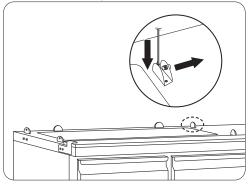
2. Insert the side glass panel into the clips. Then tighten the screws on the clips to fix the glass panel in place.
