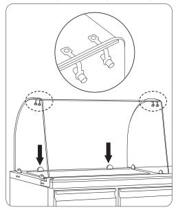
Fix the top part of the back panel in place with the supplied joint assembly. Now the sneeze guard is mounted.
