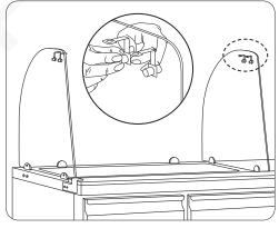
Insert the back glass panel into the clips. Then tighten the screws on the clips to fix the back panel in place. Now press gently the top part of the back panel onto the joint assembly.
