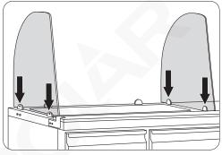
3. Mount the joint assembly onto the glass panel.
